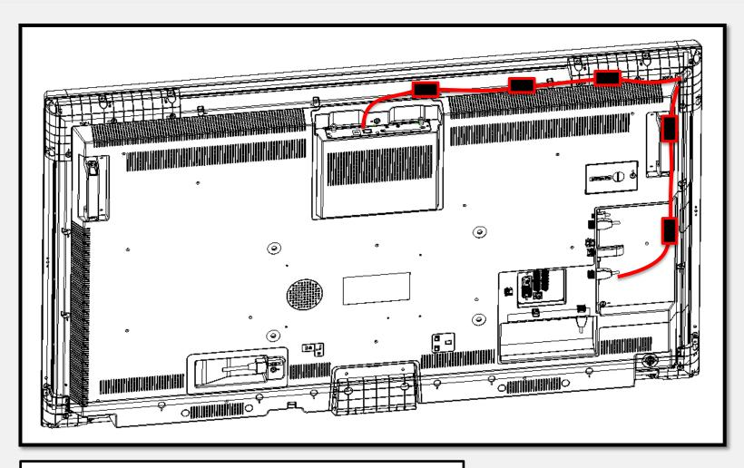
USE CABLE HOLDERS FOR CABLE POSITIONING.
